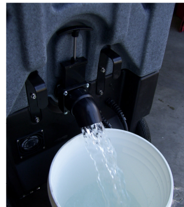
Drain water from Recovery Tank
